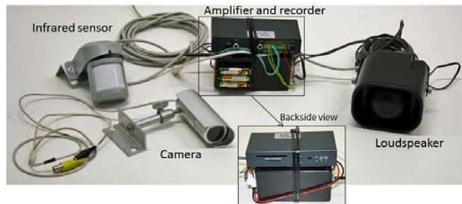
**Figure 5.4-1: Equipment for the provision of sound warnings and collection of evaluation data (excluding 12V battery).**
