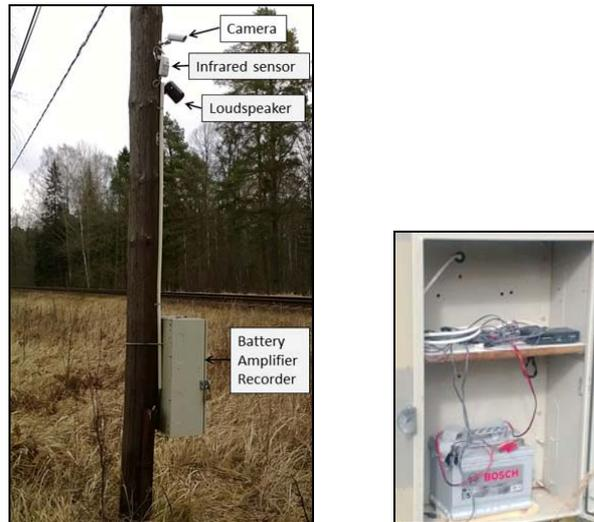
**Figure 5.4-2: Pilot test equipment at the Tammissaari site. The camera and recorder are needed only for the collection of evaluation data.**
